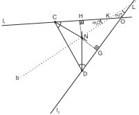
With one of the ways that were mentioned before we determine a point of the required angle bisector (for example N incenter of triangle OCD). From the point N we trace Nb//AB.
