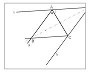
From an arbitrary point A on  $l_1$  we trace Ax//  $l_2$ . We also construct the angle bisector of OÂx, that intersects  $l_2$  at C. Then we trace from C a line parallel to  $l_1$  that cuts Ax at B. ABCO is a parallelogram because the opposite sides are parallels. Also: a diagonal (AC) bisects an angle (  $X\hat{A}O$ ), so ABCO is a rhombus. As a result, to construct the angle bisector of the required angle we
