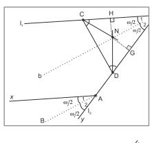
We construct a straight line  $Ax/l l_1$ , where A lies on  $l_2$ . Suppose, that O is the point of intersection of  $l_1$  and  $l_2$ . The formed angle  $x\hat{A}y$  is equal to  $l_1\hat{O}l_2 = \hat{\omega}$  as corresponding angles. We trace the angle bisector of  $x\hat{A}y$ . The considered angle bisector *b* of  $l_1\hat{O}l_2$  is parallel to AB because  $\hat{O}_2 = \hat{A}_2 = \frac{\hat{\omega}}{2}$ (corresponding angles).
