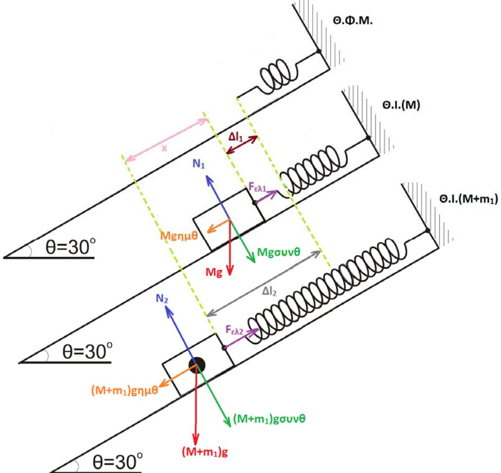
$$\Theta.I. (M) : k \cdot \Delta l_1 = Mg \cdot \eta \mu \theta \Rightarrow \Delta l_1 = \frac{Mg \cdot \eta \mu \theta}{k} = \frac{3 \cdot 10 \cdot \frac{1}{2}}{100} = 0,15 \text{ m}$$
