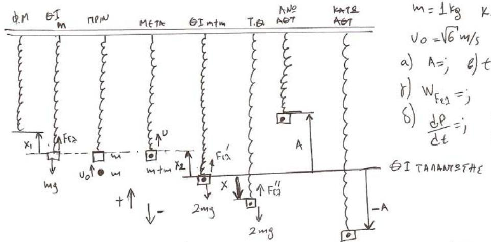
$$\underline{\text{DIN}} \quad \Sigma F = 0 \Rightarrow mg = F_G \Rightarrow mg = k \cdot x_1 \Rightarrow x_1 = \frac{mg}{k} \Rightarrow x_1 = \frac{1 \cdot 10}{100} m \Rightarrow x_1 = 0,1m$$
