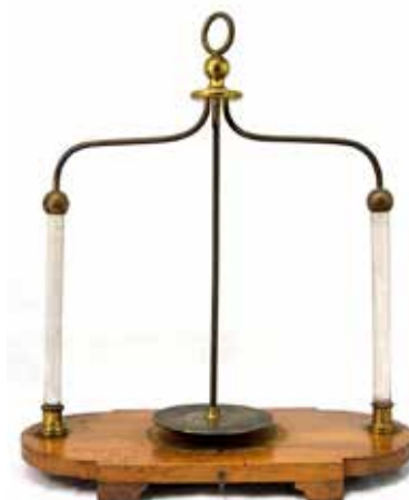
Fig. 19 Electrical Puppet Theatre, an electrostatic instruments demonstrating attraction and repulsion by means of 'dancing' pith figure (Zappeion School).
