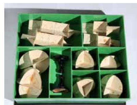
Fig. 5 Pasteboard Models for explaining the Ring Systems in uniaxial and biaxial Crystals, after Fresnel. Phanar Greek Orthodox College.
