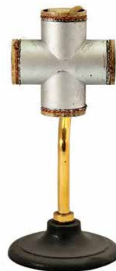
Fig. 2 Apparatus for demonstrating that atmospheric pressure acts upon all the surfaces of an object. Phanar Greek Orthodox College.
