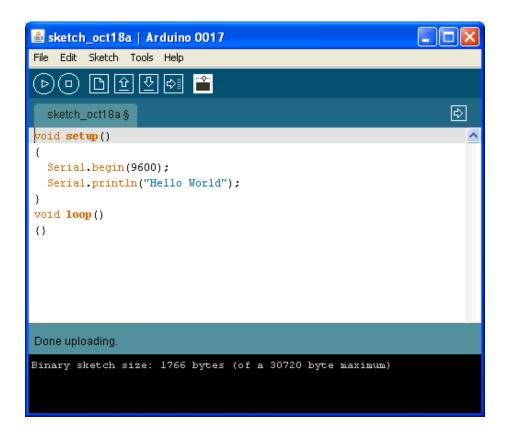
Click the Upload button or <u>Ctrl-</u>U to compile the program and load on the Arduino board.
