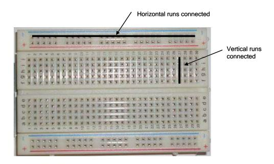
Warning: Only use solid wire on the breadboard. Strands of stranded wire can break off and fill the holes permanently.
