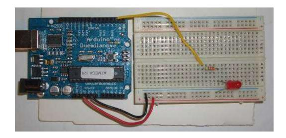
To test whether the LED works, temporarily disconnect the wire from pin 2 on the Arduino board and touch to the 5V power bus. The LED should light up. If not, try changing the orientation of the LED. Place the wire back in pin 2. On the LED, current runs from the anode (+) to the cathode (-) which is marked by the notch. The circuit you just wired up is represented in schematic form in the figure to the right.
