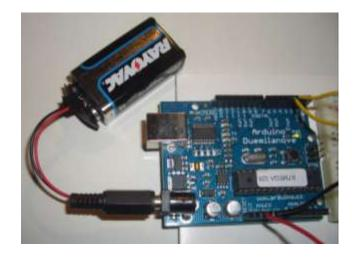
**Warning:** Watch the polarity as you connect your battery to the snap as reverse orientation could blow out your board.
