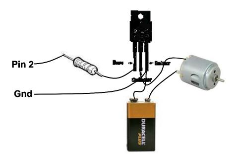
Pin 2 can be any digital I/O pin on your Arduino. Connect the minus of the battery to the emitter of the transistor (E pin) and also connect the emitter of the transistor to Gnd on the Arduino board.
