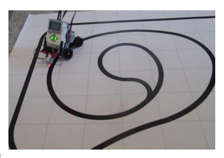
"When the sensor detects black, we will need to continuously make small correction movements forward and right, until the sensor detects white again, a.s.o. In this way, the robot keeps moving forward in a zigzag motion, its color sensor being continuously kept over the black line's right border!"
