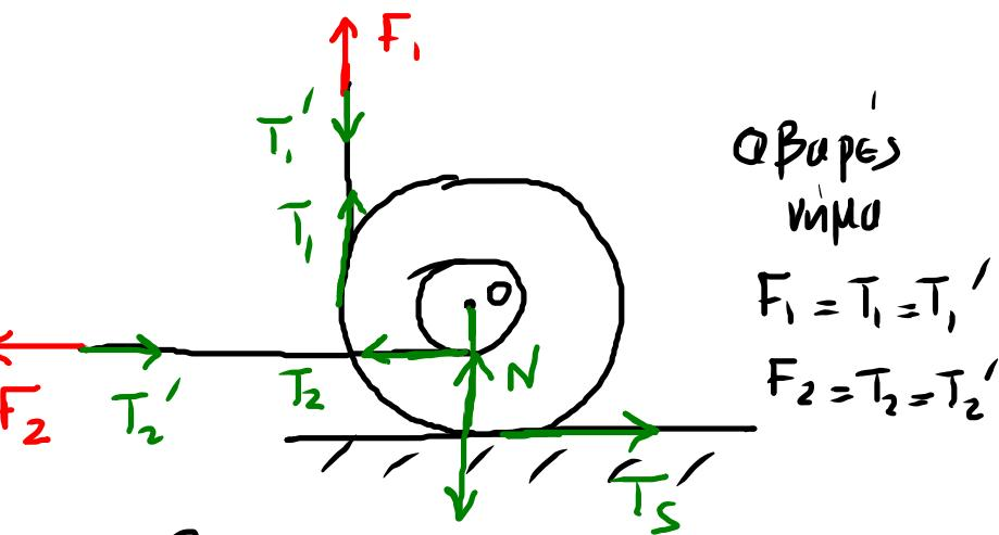
$$F_2 = F_1 + \frac{F_2}{2} \Rightarrow F_1 = \underline{\underline{\frac{F_2}{2}}}$$
