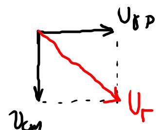
$$U_{\Gamma} = \sqrt{U_{\text{cm}}^2 + U_{\text{γρ}}^2} = \sqrt{U_{\text{cm}}^2 + (\omega R)^2} = \sqrt{U_{\text{cm}}^2 + U_{\text{cm}}^2}$$
