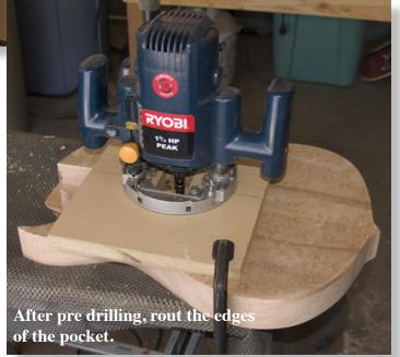
itself. The size and shape of these cavities will depend on the type of tremolo you plan on using. Hopefully, the bridge you purchased came with a schematic that shows both the dimensions and placement. If not, you'll have to do some research. I hope you took care of this early on during the design phase of your guitar. After all, now wouldn't be the time to discover you
