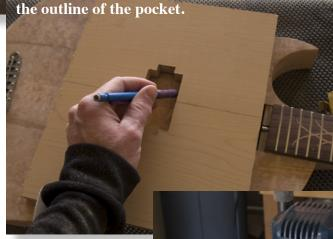
needs to be done to install a tremolo bridge. More cavities to rout! That's right, if you've opted for a tremolo, you're like going to have rout some more cavities in the body to account
