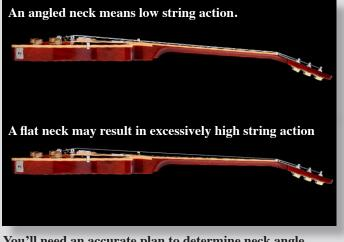
You'll need an accurate plan to determine neck angle. You could always guess based on the standard of between -1.5° and -3°, but if you're wrong, it could be impossible to fix.
