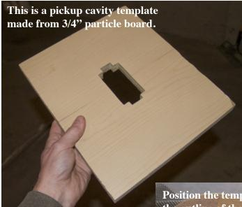
approach you used for the neck pocket. After marking their positions, drill out the cavities with a large Forstner bit. Then clamp the template into place and rout the edges with a top bearing pattern bit. It's that simple.
