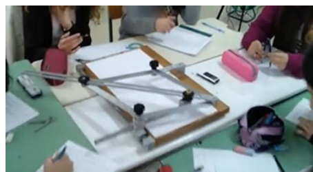
Figure 1: A van Schooten parabolograph of MML9GLP and related experimental teaching in 2022 at the 9 th General Lyceum of Patras https://www.geogebra.org/m/fafjvqkq
