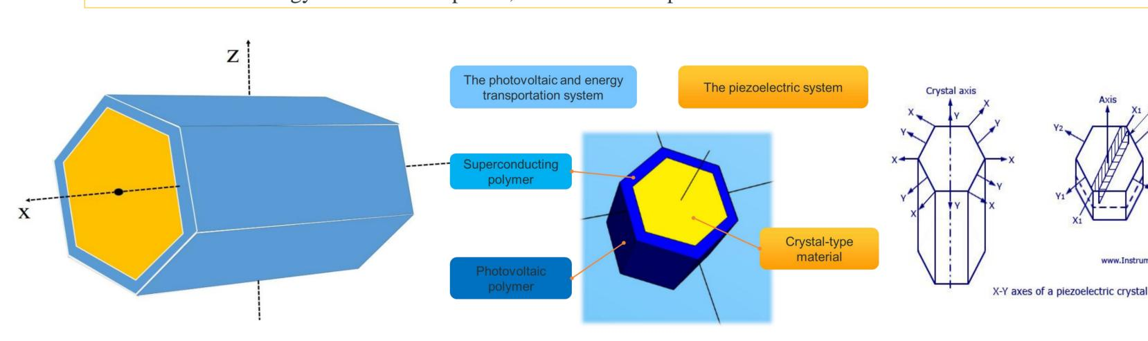
The second part lies deeper, within the second layer and consists the main and most important part of the nanosystem, its core. Here, the material used is a piezoelectric, crystal – type material. It plays its role as a "filling", as it fills up the empty space inside the nanostructure. In order to produce electrical power, the piezoelectric material needs to receive waves of mechanical energy
