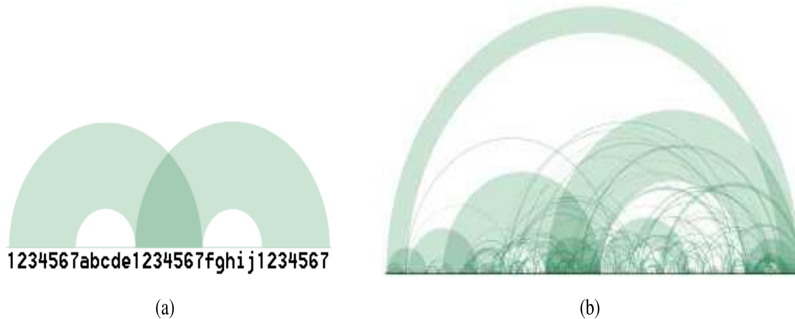
Figure 2.1: Arc Diagrams: (a) Three repeated substrings 1234567 connected by two arcs. The width of the arc is proportional to the length of the repeated subsequence while the radius is proportional to the distance between the matching pair. (b) An example illustrating Für Elise .
