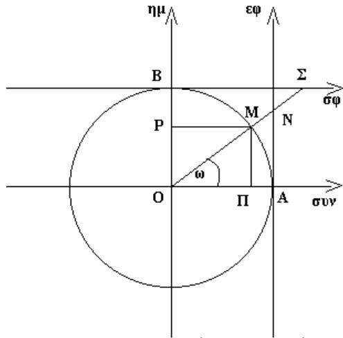
$$\sigma_{vn} = \overline{OP}, \quad \eta_{mu} = \overline{OP}, \quad \epsilon_{phi} = \overline{AN}, \quad \sigma_{phi} = \overline{BS}.$$
