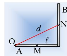
$$\text{Στερεό } \Sigma_2: I_{O2} = I_2 = I_A + I_B = \left( I_{cm} + \frac{m l^2}{4} \right) + \left( I_{cm} + m d^2 \right) \rightarrow$$
