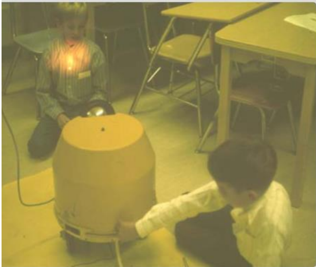
This is the first Turtle made in 1970. It was made by Tom Callahan at the MIT Lab and met Paterson's specification.
