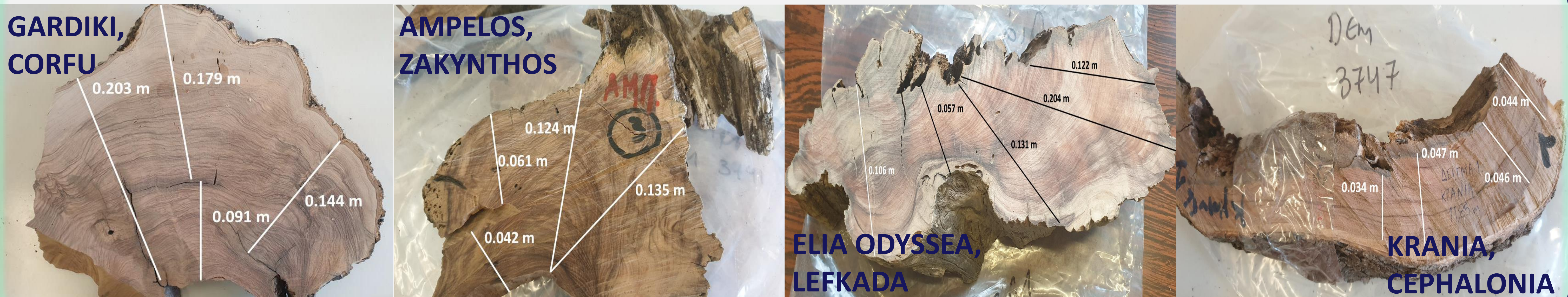
Calculation of the radial growth rate was performed using the number of rings that were counted over distances on healthy pieces of wood from each tree, assuming that this rate was stable all over the trees' lives. An average value of 0.8 – 1.2 mm/year was calculated. Ages were the ratios of radius over the radial growth rate
